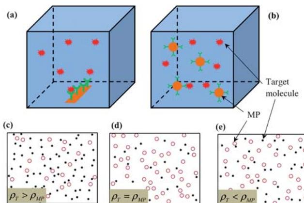
**Fig. 1** (a) Classical biosensor with the sensor at rest and waiting for the molecules to arrive on the surface. (b) Magnetic particle sensor: magnetic particles functionalized with the capture probes are distributed in the system. (c)–(e) Schematics illustrating the different regimes of bio-molecule (solid dots) detection by MPs (open circles). (c) indicates  $\rho_T > \rho_{MP}$ , (d)  $\rho_T = \rho_{MP}$ , and (e)  $\rho_T < \rho_{MP}$ .
