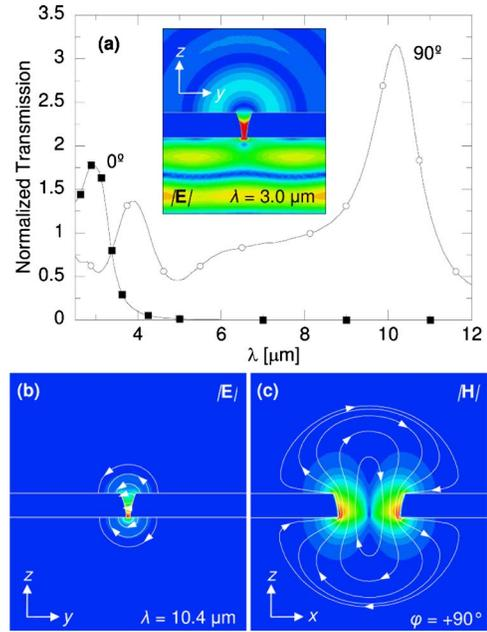
Fig. 3. (Color online) Simulated response from an isolated aperture: (a) transmission spectra, field distributions from eigenmode simulation; (b) electric field in the  $yz$  plane and (c) magnetic field in the  $xz$  plane.
