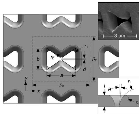
Fig. 1. Simulated geometry of focused-ion-beam (FIB) milled bowtie aperture array (not drawn to scale). Insets, an SEM image taken at  $52^\circ$  and a cross-section on the  $yz$  plane through the gap of one of the apertures.
