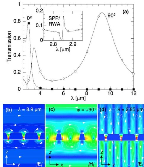
Fig. 4. (Color online) Simulation results of an array of bowtie apertures: (a) transmission spectra with close-up of SPP/RWA in inset, (b) electric field in the  $yz$  plane (c) magnetic field in the  $xz$  plane, both for the TE<sub>10</sub> mode, and (d) electric field on the  $yz$  plane for the SPP/RWA.
