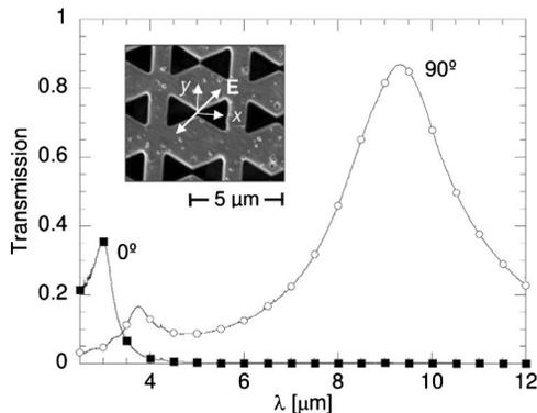
Fig. 2. Experimental results for the normally illuminated bowtie aperture array at  $0^\circ$  and  $90^\circ$  polarizations. The inset is an SEM image of the array.
