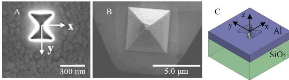
Fig. 2. (A) SEM image of the bowtie nano-aperture on a 150nm coated Al film. The aperture has a size of  $260 \text{ nm} \times 260 \text{ nm}$  and has a gap of 62 nm. (B) SEM image of the NSOM probe. The hole on the tip is around 150 nm in diameter. (C) Simulation model of bowtie nano-antenna. Its dimensions used in simulation are fit to SEM image (A).
