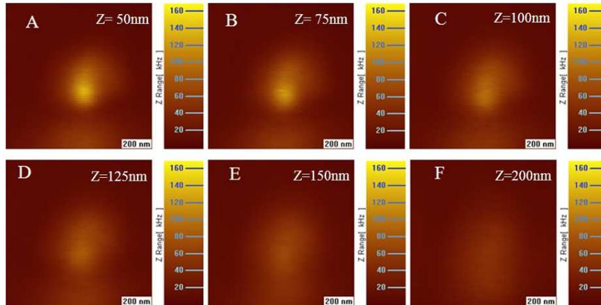
Fig. 7. Constant-height scanning NSOM images at different tip-sample distances: 50 nm, 75 nm, 100 nm, 125 nm, 150 nm and 200 nm in A - F, respectively. The laser polarization is in the x-direction.
