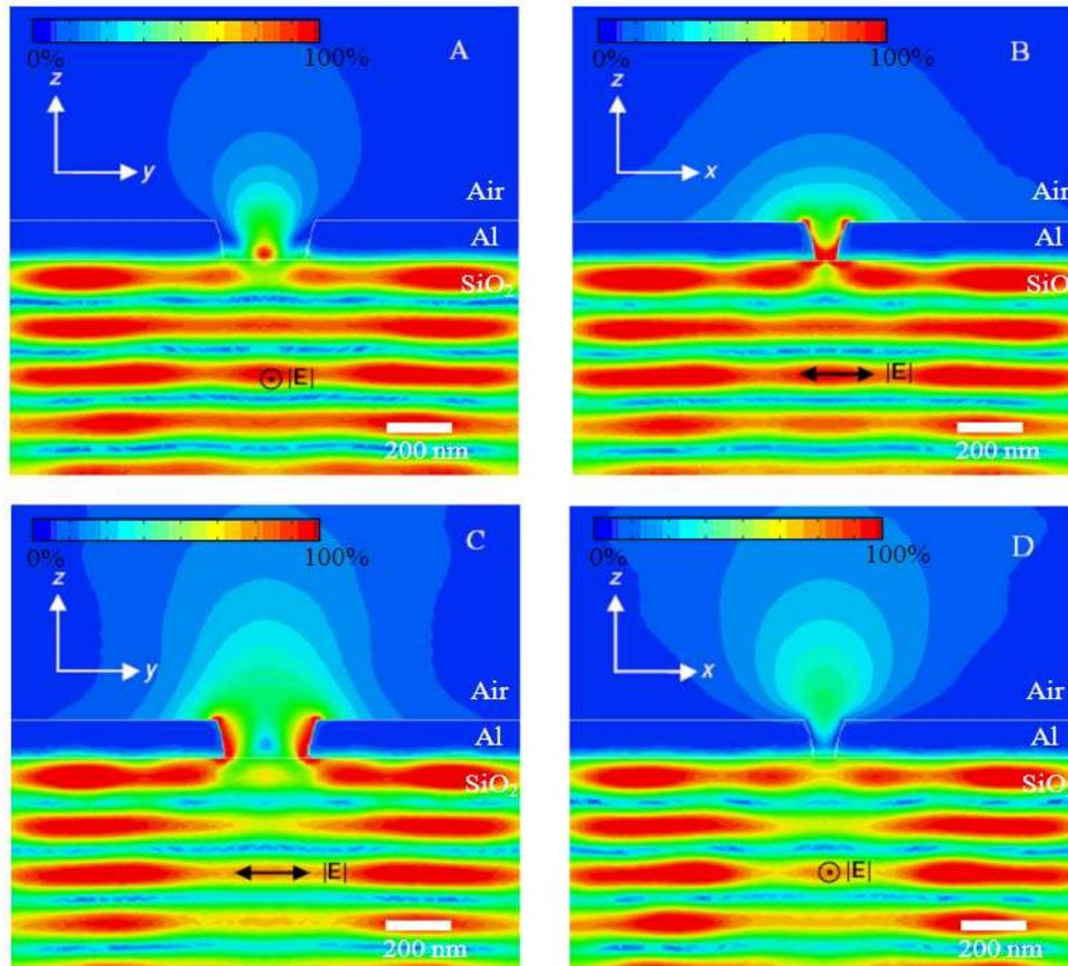
Fig. 3. Computed electric field distribution of bowtie aperture under x-polarized illumination (A, B) and y-polarized illumination (C, D). The aperture has a size of 260 nm  $\times$  260 nm and a gap of about 62 nm at the fused silica/aluminum interface and 134 nm at the top of the film. The illumination is a  $\lambda = 457$  nm plane-wave.
