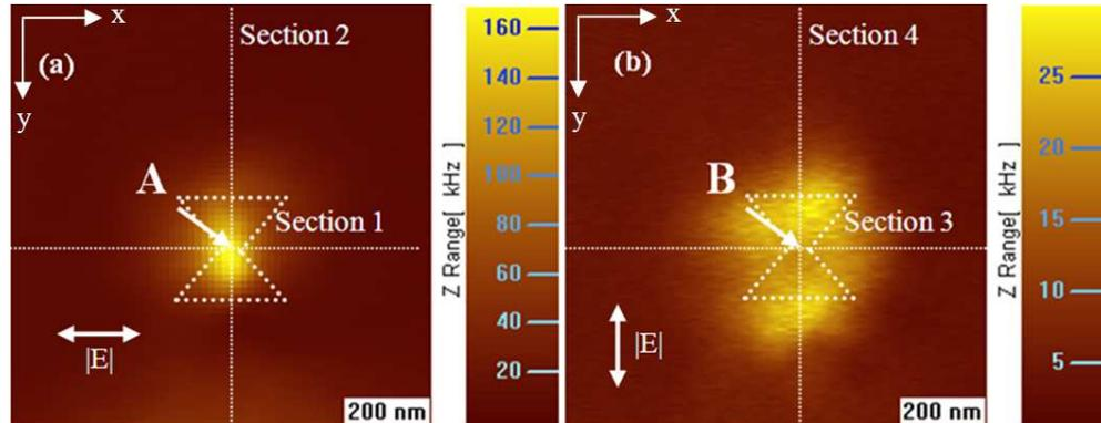
Fig. 4. Near-field intensity distribution of bowtie aperture measured in the contact mode. The scan area is  $1\mu\text{m} \times 1\mu\text{m}$ . The illumination laser is polarized along the x-direction (A) and y-direction (B). Note the different intensity scales in the two figures.
