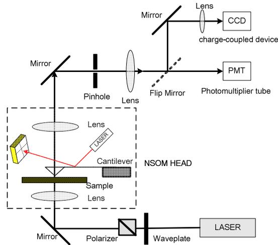
Fig. 1. Schematic of home-made NSOM system. The illumination source is a  $\lambda = 457$  nm argon-ion laser. The feedback of NSOM head is based on the optical beam deflection technique. The NSOM probe is an aluminum coated  $\text{Si}_3\text{N}_4$  probe with a 150 nm hole at the tip. The pinhole has a size of 100 micron.
