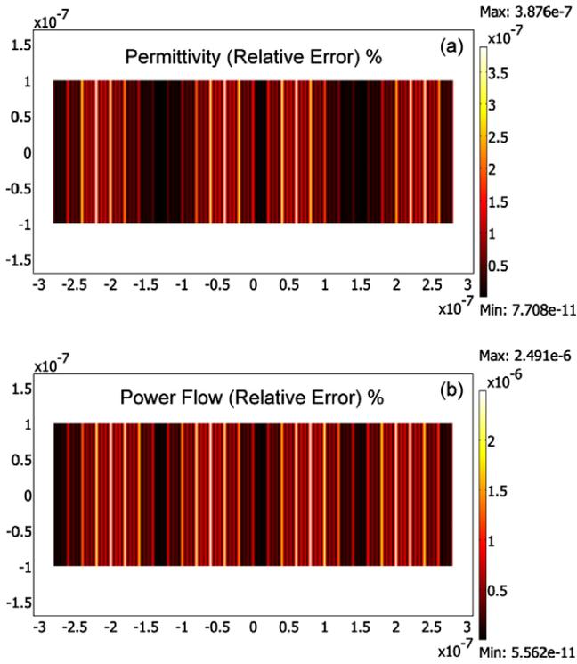
**Fig. 1.** Validation of the FE scalar  $H$ -field models. (a) Relative error in time-averaged  $\epsilon$  of a 560-nm thick non-linear Kerr slab ( $\epsilon_i = 2.25$  and  $\chi^{(3)} = 10^{-18} \text{ m}^2/\text{V}^2$ ) with effective  $\epsilon$  obtained from (19). (b) Relative error in time-averaged power flow through the slab calculated using scalar  $H$ -field formulation with effective  $\epsilon$  also obtained from (19).
