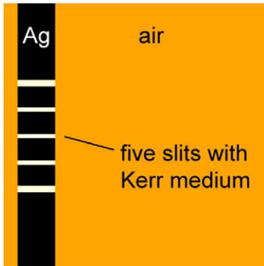
**Fig. 2.** Geometry of a non-linear focusing device. A 570-nm thick silver film is illuminated by 850-nm plane wave moving from left to right through five sub-wavelength slits (with 100-, 70-, 60-, 70-, 100-nm width sequence) distributed evenly from top to bottom with 400-nm offsets between their centers.
