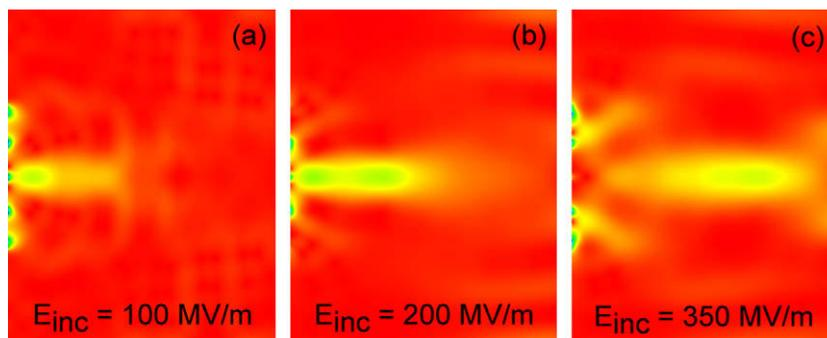
**Fig. 4.** Intensity-tunable focusing at the incident magnitude of 100 MV/m (a), 200 MV/m (b), and 350 MV/m (c).
