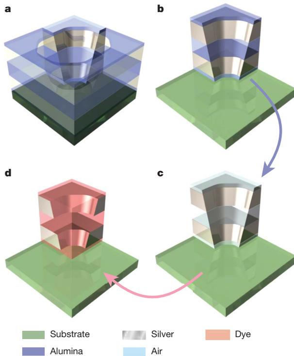
**Figure 1 | Schematic of the fabrication process.** **a**, Unit cell of the fishnet structure with alumina as the spacer material between two silver layers. **b**, One-quarter of the fishnet structure with an alumina spacer. **c**, After etching the alumina, the fishnet structure has air or solvent as the spacer with alumina pillars as support. **d**, After coating with Rh800-epoxy, the fishnet structure has the dye-epoxy material in the spacer region and above the fishnet structure.
