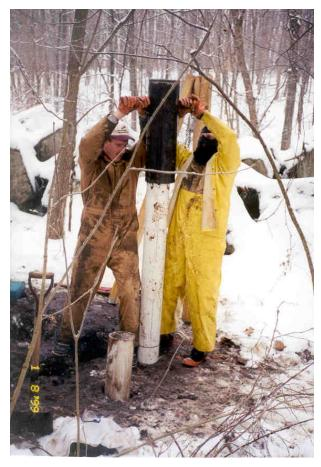
Figure 2. Soil sampling for site characterization for phytoremediation site clean-up in Bedford, Indiana.
