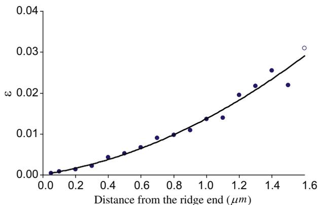
**Fig. 9** – The strain in a secondary ridge of an FLG sample grown at 1550 °C on 4H–SiC as a function of length. The solid line is the result of a least-squares fit.
