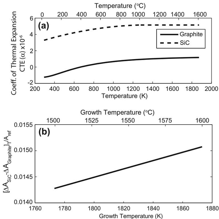
**Fig. 6** – In (a), the coefficient of thermal expansion of the basal plane of 4H-SiC(000 $\bar{1}$ ) (dashed line, Ref. [32]) and the basal plane of graphite (solid line, Ref. [31]). For temperatures greater than 1000 °C the coefficient of thermal expansion of 4H-SiC is assumed to be constant. In (b), the predicted fractional change in area between SiC and graphite when cooled from a specific growth temperature to room temperature (20 °C).
