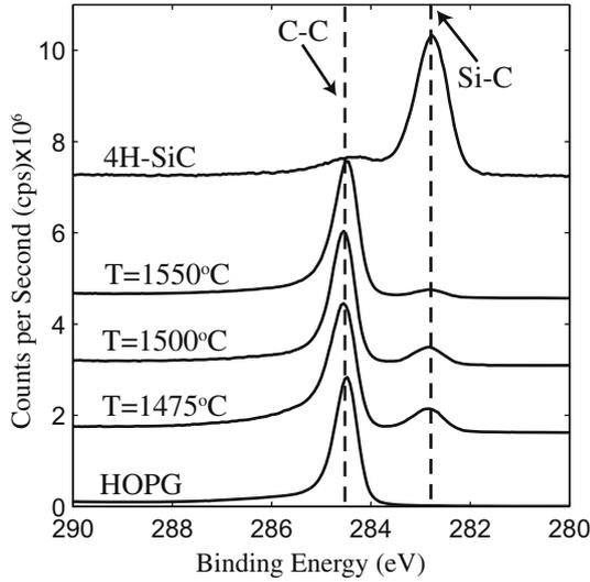
**Fig. 1** – Comparison of the C 1s spectra taken from different samples at 0° photoemission angle. The XPS spectrum from HOPG identifies the binding energy of the  $sp^2$  C–C bond XPS spectrum. Data for FLG grown for ten minutes at temperatures of 1475, 1500, and 1550 °C show a reduced C–Si signal as the FLG thickness increases. A representative C 1s spectrum from SiC is also provided. Each spectrum is shifted upward by a constant offset for purposes of clarity.
