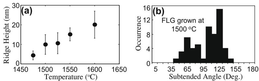
**Fig. 5** – In (a), the average height of ridges in FLG samples plotted as a function of the growth temperature. In (b), a histogram plot of the subtended angle between ridges for the FLG sample grown at 1500 °C.
