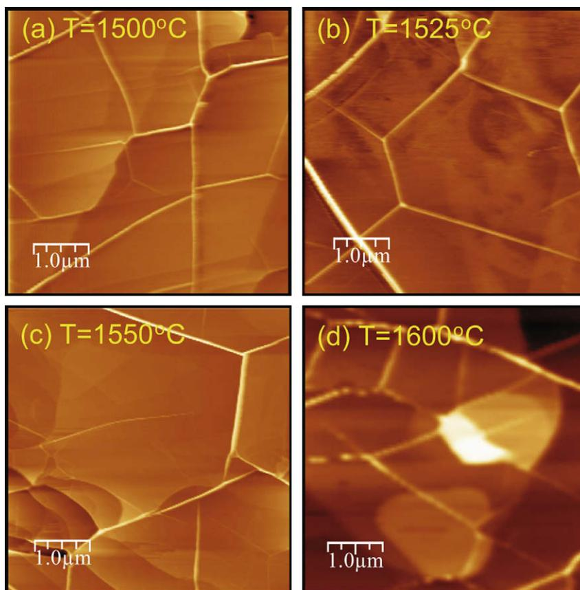
Fig. 3 – A comparison between  $5\ \mu\text{m} \times 5\ \mu\text{m}$  AFM images of FLG grown on 4H-SiC(0001) substrate at growth temperatures of (a)  $T_G = 1500\ \text{°C}$ , (b)  $T_G = 1525\ \text{°C}$ , (c)  $T_G = 1550\ \text{°C}$ , and (d)  $T_G = 1600\ \text{°C}$ . All samples were held at the specified growth temperature for 10 min.
