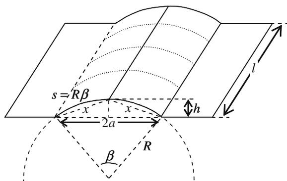
Fig. 7 – Schematic of a ridge structure showing the relevant parameters for estimating the excess area.
