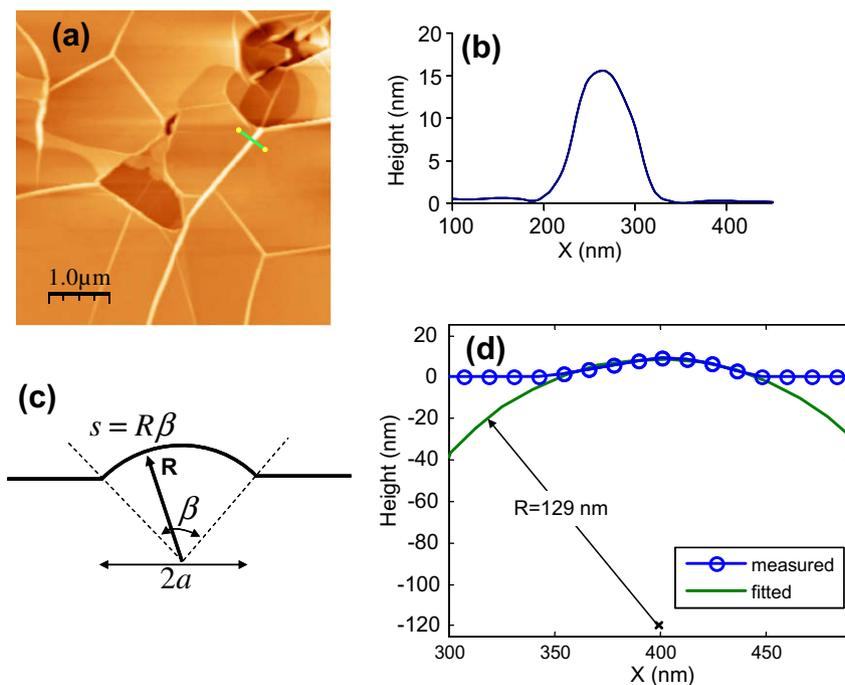
Fig. 8 – In (a), an AFM image of primary ridges on FLG grown at 1550 °C on 4H-SiC. In (b), the cross-sectional line profile along the line in (a). In (c), a schematic cross-section of a ridge of width  $2a$ . In (d), the results of a least-squares fit of the ridge profile to a circle. The radius of curvature of the ridge is found to be 129 nm.
