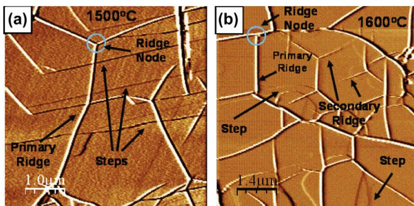
Fig. 4 – In (a), the derivative of a typical AFM image obtained from FLG grown at  $1500\ \text{°C}$  for 10 min. In (b), the derivative of a typical AFM image obtained from FLG grown at  $1600\ \text{°C}$  for 10 min.
