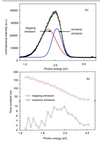
**Figure 5.** (a) The luminescence spectrum of CdS:Te QDs with a Te/S molar ratio of 1.1%. It can be decomposed into a higher-energy component (blue) due to excitonic emission and a lower-energy component due to trapping state emission (red). (b) Lifetime of the excitonic and trapping state emissions as a function of photon energy.
