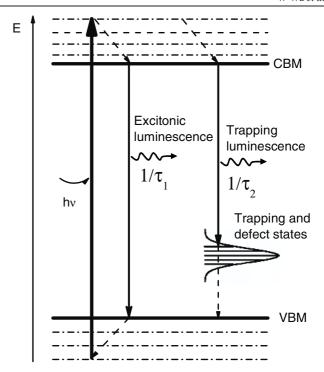
**Figure 4.** Energy level diagram of CdS:Te QDs, where trapping and defect states are shown. CBM, conduction band minimum; VBM, valance band maximum.
