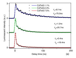
**Figure 6.** Normalized luminescence decay curves of three CdS:Te QD samples at 400 nm laser excitation. The decays of three different CdS:Te QDs are integrated about 30 nm near the emission peak.
