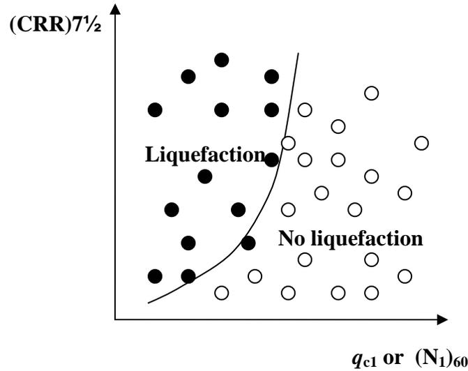
Figure 4 – Semi-empirical approach to evaluate liquefaction resistance.
