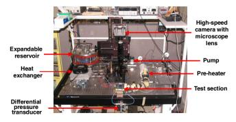
Fig. 1. Photograph of the experimental facility.
