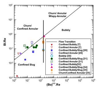
**Fig. 8.** Comparison of the comprehensive flow regime map with the experimental data from the literature.
