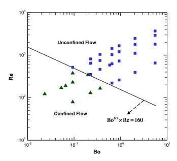
Fig. 4. Transition from confined flow to unconfined flow.
