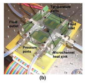
Fig. 2. (a) Microchannel test chip and (b) test section assembly.
