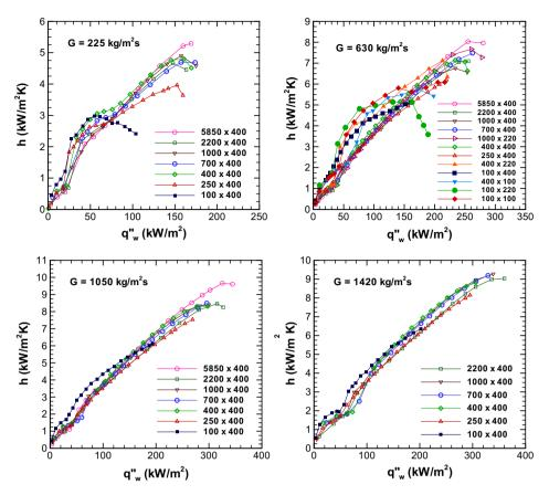
Fig. 6. Effects of physical confinement on heat transfer coefficients for four mass fluxes; the microchannel dimensions are presented as width  $(\mu m) \times \text{depth}$  ( $\mu m$ ).
