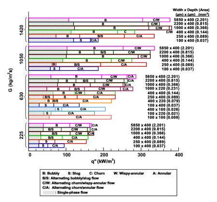
Fig. 3. Summary of boiling flow patterns in the microchannel test pieces; the microchannel dimensions are presented as width  $(\mu m) \times depth (\mu m)$  with a single-channel cross-sectional area  $(mm^2)$  in parentheses.
