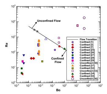
**Fig. 5.** Comparison of the confinement criterion with experimental data from a variety of sources in the literature.
