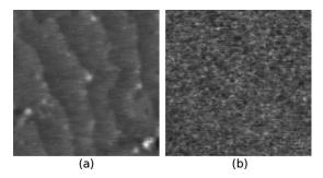
FIG. 2.  $1\times1~\mu\text{m}^2$  AFM images of lightly doped (a) and heavily doped (b) hydrogen-terminated silicon wafers. The steps in (a) correspond to individual planes of Si atoms. The root-mean-square roughnesses of the images are 1.1 and 1.6 Å, respectively.
