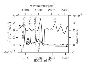
FIG. 14. Comparison of infrared and inelastic electron tunneling spectroscopies of Au/N-benz/Si structures.
