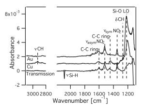
FIG. 13. Infrared spectra of as deposited (transmission) and metallized N-benz on Si. Cu significantly alters the molecular spectrum, whereas molecular features are preserved after Au deposition.
