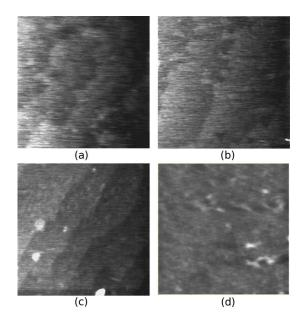
FIG. 3. (Color online) AFM images of B-benz (a), D-benz (b), M-benz (c), and N-benz (d) on *n*-type Si. Atomic step edges are still visible in (a)–(c), whereas (d) exhibits much less-ideal topography.
