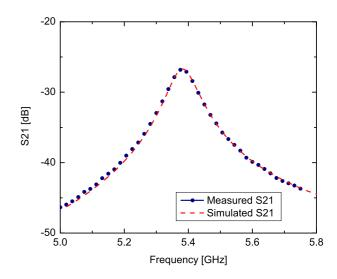
Fig. 5. Measured and simulated power transmission for the 10mm liquid metal resonator.
