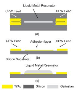
Fig. 1. Design of the liquid metal microstrip resonator:(a)Top view;(b)Side view with only the Ti/Au layer;(c)Side view with liquid metal resonator.
