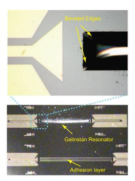
Fig. 2. Picture of the fabricated Galinstan resonator.
