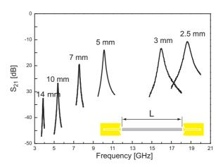
Fig. 3. Measured S<sub>21</sub> of weakly coupled Galinstan resonators.
