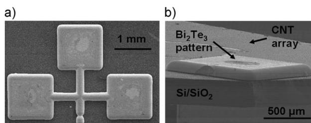
**Figure 3.** FESEM images showing a) top view of a  $\text{Bi}_2\text{Te}_3$  pattern electrodeposited on top of a CNT array and b) side view of a thick  $\text{Bi}_2\text{Te}_3$  pattern on CNT array.
