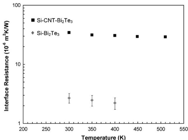
**Figure 4.** Thermal interface resistance as a function of interface temperature measured using the PA technique. The error in the interface resistance measurements is  $\pm 1 \text{ m}^2 \text{ K W}^{-1}$  and too small to appear on the log-scale for the larger resistance values.
