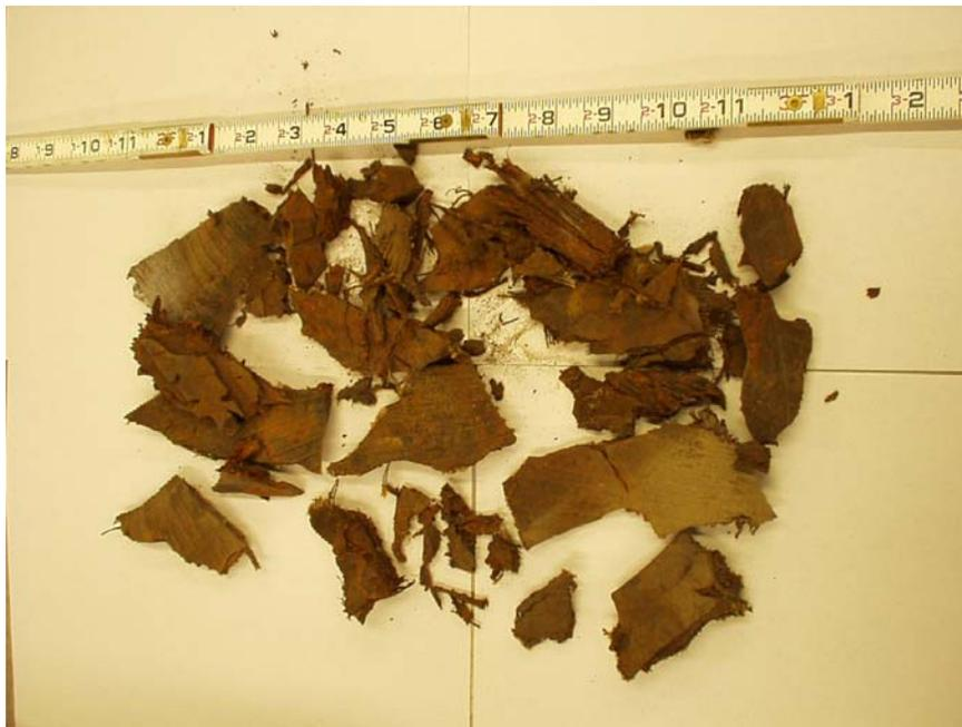
**Figure 3.1 Tire Shreds Used for the Embankment**
