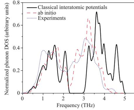
FIG. 2. (Color online) Normalized phonon density of states of  $\text{Bi}_2\text{Te}_3$  with respect to frequency. Heavy solid curve: computed classical interatomic potentials; light dashed curve: computed *ab initio*; dashed curve: experimental values from Ref. 20.
