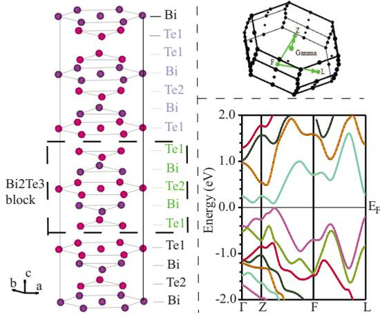
FIG. 1. (Color online) Left:  $\text{Bi}_2\text{Te}_3$  hexagonal conventional cell structure; upper right:  $\text{Bi}_2\text{Te}_3$  first Brillouin zone; lower right:  $\text{Bi}_2\text{Te}_3$  electronic band structure along some high-symmetry lines.
