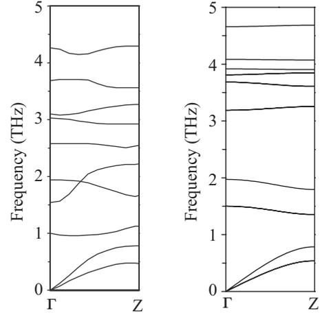
FIG. 3. Phonon dispersion of  $\text{Bi}_2\text{Te}_3$  computed using classical interatomic potentials along high-symmetry direction  $\Gamma$ -Z (right) compared to experimental phonon dispersion from Ref. 20 (left).
