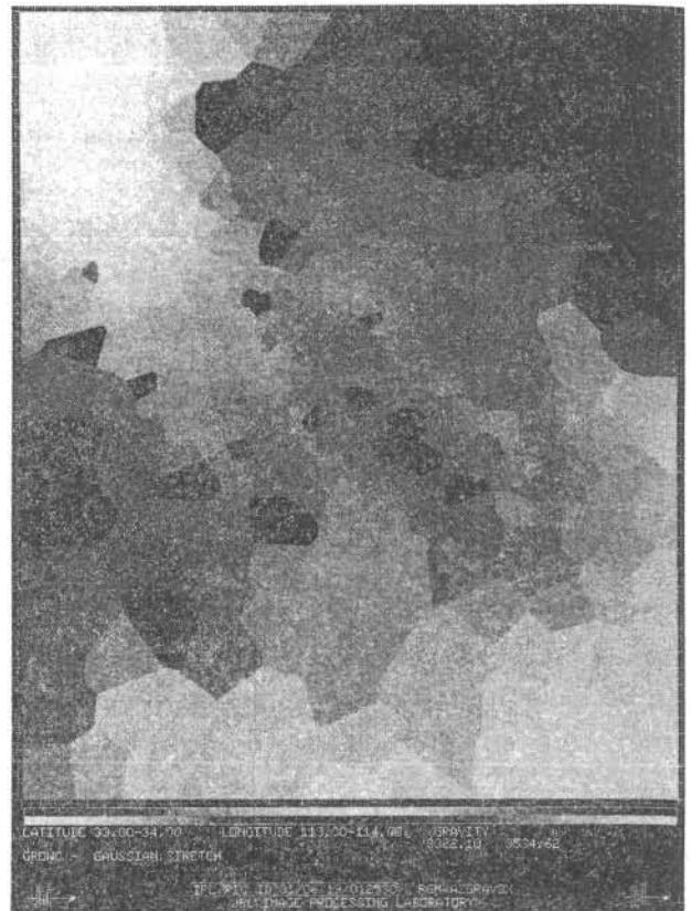
Figure 5: Interpolated Gravity Image. This image, for the Phoenix West Quad shows the faceted gravity data. The data were a set of points distributed somewhat randomly throughout the quad and were "grown" until all converged. The brightness of each grey tone corresponds to the intensity of gravity. These data were rotated and scaled to register with the Landsat quad.
