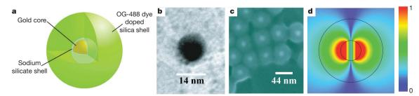
**Figure 1** | **Spaser design. a**, Diagram of the hybrid nanoparticle architecture (not to scale), indicating dye molecules throughout the silica shell. **b**, Transmission electron microscope image of Au core. **c**, Scanning electron microscope image of Au/silica/dye core–shell nanoparticles. **d**, Spaser mode
