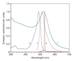
**Figure 2** | **Spectroscopic results.** Normalized extinction (1), excitation (2), spontaneous emission (3), and stimulated emission (4) spectra of Au/silica/dye nanoparticles. The peak extinction cross-section of the nanoparticles is  $1.1 \times 10^{-12} \, \mathrm{cm}^2$ . The emission and excitation spectra were measured in a spectrofluorometer at low fluence.
