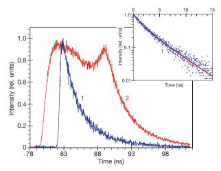
**Figure 3** | **Emission kinetics.** Main panel, emission kinetics detected at 480 nm (1) and 520 nm (2). Inset, trace 1 plotted in semi-logarithmic coordinates (dots) and the corresponding fitting curve. The beginning of each emission kinetic trace coincides with the 90-ps pumping pulse.
