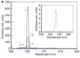
**Figure 4** | **Stimulated emission.** a, Main panel, stimulated emission spectra of the nanoparticle sample pumped with 22.5 mJ (1), 9 mJ (2), 4.5 mJ (3), 2 mJ (4) and 1.25 mJ (5) 5-ns optical parametric oscillator pulses at  $\lambda = 488$  nm. b, Main panel, corresponding input–output curve (lower axis, total launched pumping energy; upper axis, absorbed pumping energy per nanoparticle); for most experimental points,  $\sim$ 5% error bars (determined
