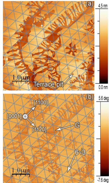
FIG. 6. (Color online) Images of AFM (a) topography and (b) phase of a 1475 °C sample held at temperature for 10 min showing preference for erosion of steps and terrace pits along the  $\{11\bar{2}0\}$  planes. Reference grid is overlaid to guide the eye along the  $\{11\bar{2}0\}$  set of planes. Phase contrast in (b) demarcates regions of graphene, labeled as G, and regions of reconstructed SiC.
