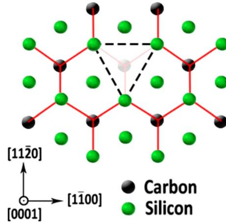
FIG. 4. (Color online) The basal plane of an unreconstructed Si face 4H-SiC surface is shown with solid lines representing the  $sp^3$  bonds characteristic of SiC. A point defect caused by the vacancy of a carbon atom is outlined by the dashes. This vacancy lowers the number of bonds along the  $\{11\bar{2}0\}$  planes which are represented by the dashed triangle.
