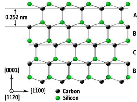
FIG. 1. (Color online) Bulk 4H-SiC crystallographic structure along the  $(11\bar{2}0)$  plane. The horizontal lines cutting across the carbon atoms are guides representing the periodic spacing between bilayers. The repeating ABC letters represent the periodic stacking structure unique to the 4H-SiC polytype.
