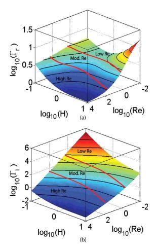
FIG. 2. (Color online) Hydrodynamic function  $\Gamma$  as a function of the unsteady Reynolds number, Re, and the nondimensional gap, H, computed based on the Tuck–Green theory. (a) shows the real part of  $\Gamma$  and (b) shows the imaginary part of  $\Gamma$ . The red lines divide the parameter space into regions of high, moderate, and low Re.
