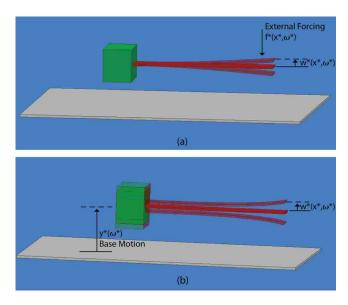
FIG. 3. (Color online) Two different excitation mechanisms for which the semianalytical expression for  $\Gamma$  can be used to predict the FRF. In (a) the microcantilever is held at a fixed distance from a rigid wall, and is excited by means of external fields such as magnetic or electrostatic forces as in magnetic mode AFM and RF switches. In (b) the microcantilever is excited inertially by means of a dither piezo at its base, as in acoustic mode AFM.
