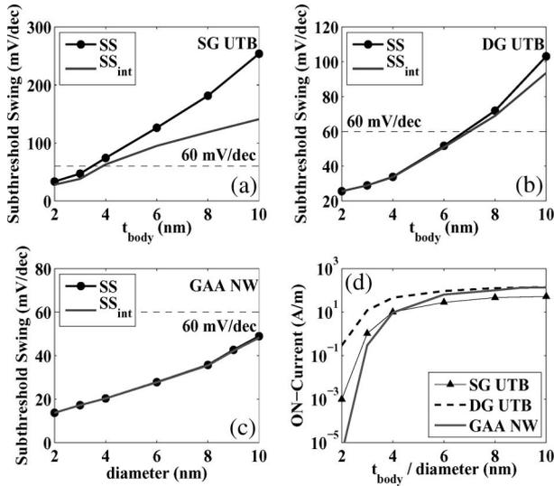
Fig. 3. (a) (Line with circles) Total (SS) and (gray line) intrinsic (SS<sub>int</sub>) SSS of the SG UTB device with different body thicknesses  $t_{\text{body}}$ 's. (b) Same as (a) for the DG UTB device. (c) Same as (a) and (b) for the GAA NW device. (d) ON current  $I_d$  at  $V_{\text{ds}} = 0.2$  V and  $V_{\text{gs}} = 0.2$  V as a function of SG UTB, DG UTB, and GAA NW device dimensions.
