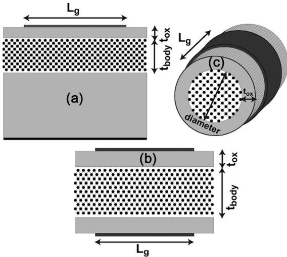
Fig. 1. Structure of the p-i-n InAs BTBT transistors considered in this letter. (a) SG UTB. (b) DG UTB. GAA NW. Devices (a) and (b) are characterized by a body thickness  $t_{\text{body}}$  ranging from 2 to 10 nm, and device (c) is characterized by a diameter  $d$  ranging between 2 and 8 nm. The gate length  $L_g = 20$  nm and “oxide thickness”  $t_{\text{ox}} = 1$  nm have the same dimensions in all three cases.
