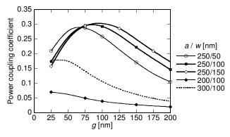
Fig. 3. Coupling efficiency from a far field light source to the waveguide. The far field light source is assumed to be a diffraction limited spot incident on the bowtie aperture with a diameter of 945.5 nm. For the bowtie aperture, a = b is used. s = d = 25 nm, f = 100 nm, and t = 50 nm.
