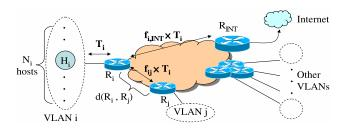
**Figure 3:** Inter-VLAN traffic sent by a host in VLAN i.
