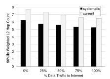
Figure 7: Reduction of hops traversed by data traffic using our systematic router placement, with varying f.
