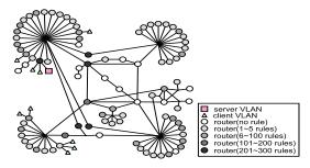
Figure 10: L3 topology showing systematic distribution of ACL rules after applying fine-gained, LB placement strategy.
