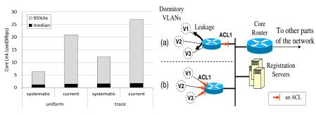
**Figure 8:** Data traffic load on core links using the uniform and the trace traffic model, with f=50.
