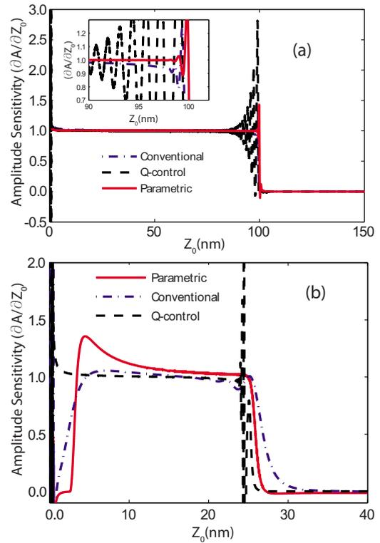
FIG. 6. (Color online) A comparison between the calculated amplitude sensitivity ( $\partial A / \partial Z_0$ ) for different types of microcantilever excitations at two different feedback gains. The calculations were performed for a Si tip approaching an HOPG sample. In (a), a feedback gain,  $G=1.0139G_{\text{th}}$ . The inset provides an expanded view of the transient behavior. In (b), a feedback gain,  $G=1.0041G_{\text{th}}$ .
