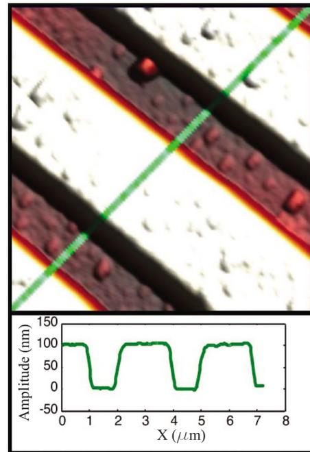
FIG. 11. (Color online) An AFM image of a MikroMasch silicon grating (TGZ02) imaged by a parametric AFM with an amplitude set-point ratio of  $0.6A_{\text{rms}}$ . Scan rate is 1.0 Hz. The figure demonstrates that at typical scan rates, there are minimal ringing transients at the edges in spite of a high  $Q_{\text{eff}}=1550$ . The image size is  $5 \times 5 \mu\text{m}^2$ . A topographic profile along the diagonal line is shown in the inset.
