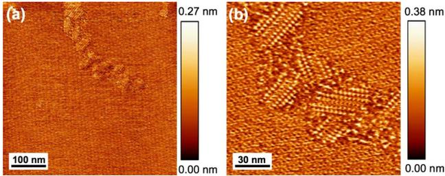
FIG. 3. (Color online) STM images of a region from the graphene grown at 1500 °C. In (a), a  $500 \times 500 \text{ nm}^2$  image showing the presence of a grain boundary in the upper half of the image. In (b), a  $150 \times 150 \text{ nm}^2$  image showing the parallel 1D features within the grain boundary. Scan parameters are  $I_{\text{set}}=2.0 \text{ nA}$  and  $V_{\text{bias}}=100 \text{ mV}$  for (a) and (b).
