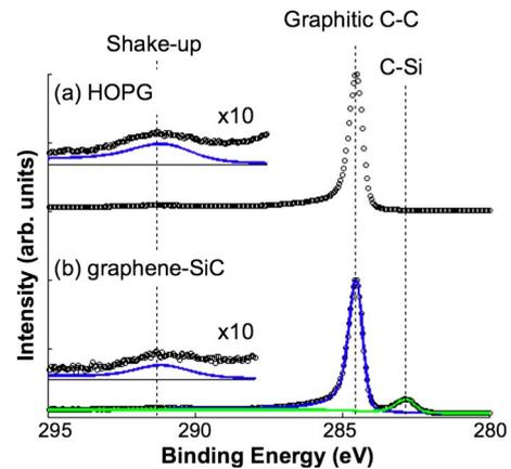
FIG. 1. (Color online) The C 1s XPS spectra, collected at  $\theta = 0^\circ$ , (a) from a reference HOPG substrate and (b) from a FLG sample grown at 1500  $^\circ$ C on SiC. The similarity of the two XPS spectra indicates the presence of graphitic carbon on SiC. Both spectra were obtained at a photoemission angle of  $0^\circ$ . A closer examination of the region between 288 and 295 eV from both samples provides evidence for shake-up satellites (insets).
