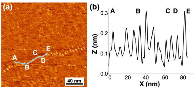
FIG. 4. (Color online) (a) An STM image of a  $200 \times 200 \text{ nm}^2$  region shows a 1D superlattice. (b) A line profile along the line  $ABCDE$ , which follows the profile of the 1D superlattice. Scan parameters are  $I_{\text{set}}=2.0 \text{ nA}$  and  $V_{\text{bias}}=300 \text{ mV}$ .
