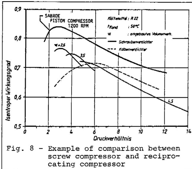
While we will readily admit that it is possible to find reciprocating compressors with very poor efficiencies, we state, that a modern, well designed reciprocating compressor should offer isentropic efficiency somewhat like the heavily traced curve, which happens to be a SABROE compressor at 1200 rpm. It should be mentioned, that there are 2 or 3 competing makes which are approximately on the same level.
