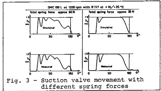
Fig. 3 - Suction valve movement with different spring forces
