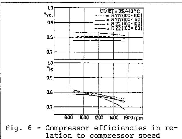
Fig. 6 - Compressor efficiencies in relation to compressor speed
