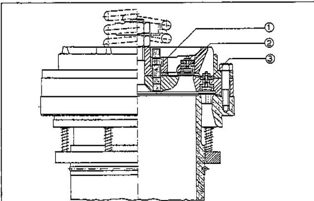
Fig. 2 - Cylinder liner with electronic pick-ups
