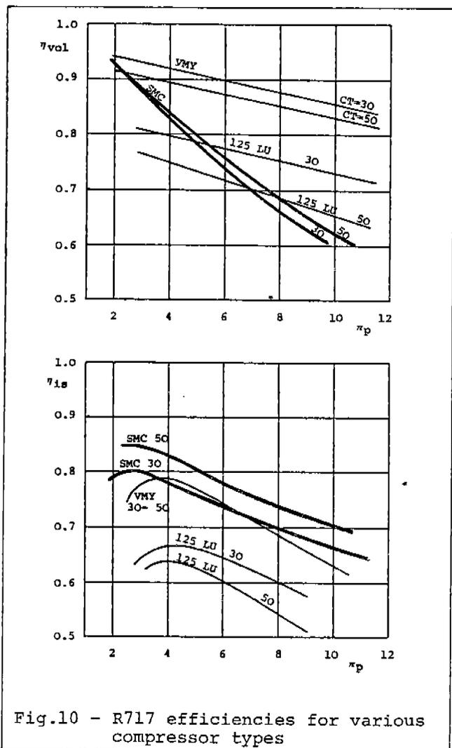
Fig.10 - R717 efficiencies for various compressor types
