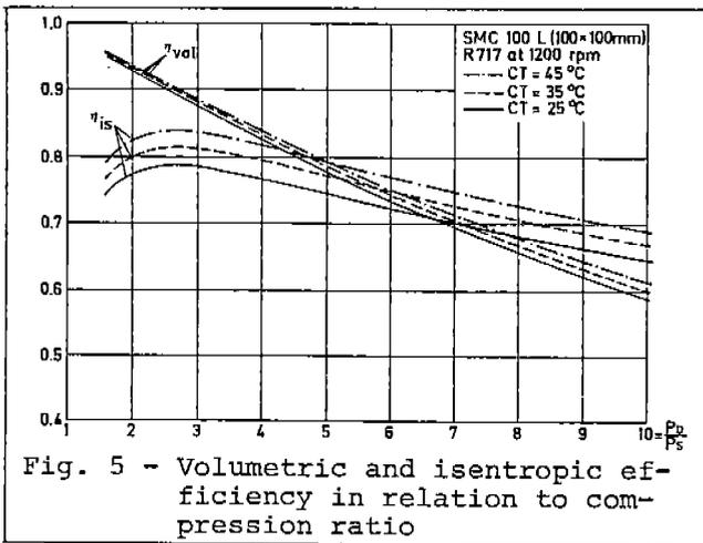
Fig. 5 - Volumetric and isentropic efficiency in relation to compression ratio
