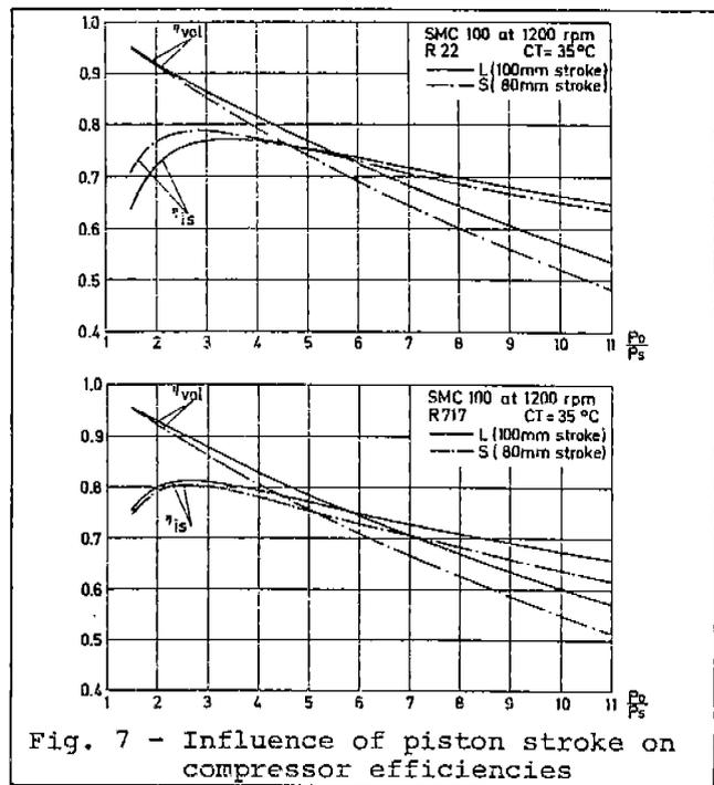
Fig. 7 - Influence of piston stroke on compressor efficiencies
