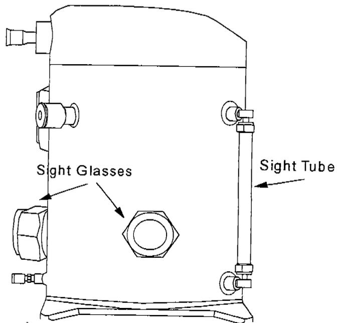
Figure 1 Compressor fitted with sight glasses and sight tube
