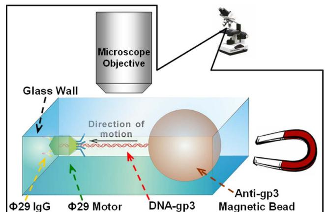
FIG. 1. (Color online) Schematic of the magnetomechanical system for bright-field analysis of phi29 DNA packaging.
