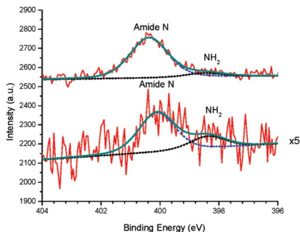
**Figure 3.** High-resolution XPS spectra of the N 1s region; (1) InP surface patterned by microcontact printing and (2) InP surface patterned by DPN. In both cases the peptide was used as an ink. The intensity difference between the two sets of data is due to a different adsorption area.
