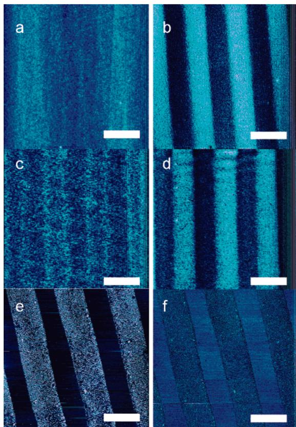
**Figure 1.** InP surfaces patterned with ODT (a and b), MHL (c and d), and peptide (e and f) using microcontact printing. The images on the left are height and on the right LFM. All images were collected using clean tips. The scan sizes were  $20\ \mu\text{m} \times 20\ \mu\text{m}$ , and the scan speed was 4.07 Hz. The scale bar is  $5\ \mu\text{m}$ .
