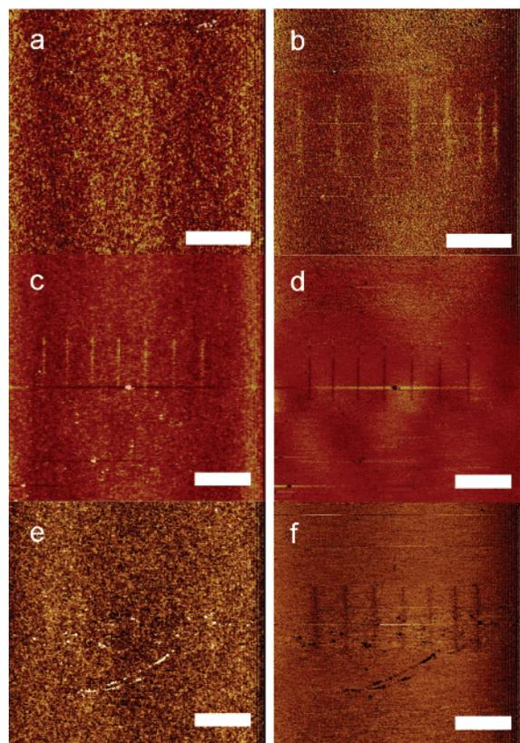
**Figure 2.** InP surfaces patterned with ODT (a and b), MHL (c and d), and peptide (e and f) using DPN. The images on the left are height and on the right LFM. All images were collected using clean tips. The scan sizes were  $20\ \mu\text{m} \times 20\ \mu\text{m}$ , and the scan speed was 3.59 Hz. The scale bar is  $5\ \mu\text{m}$ .
