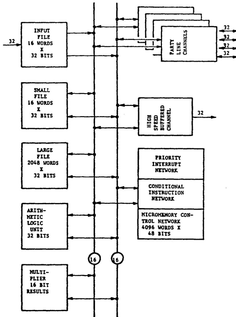
Figure 3. Data path organization in the CDC Flexible Processor<sup>10</sup>.
