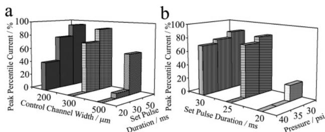
**Figure 3.** (a) Peak percentile current as a function of the control channel width and the set pulse duration (the pulse duration designated by our control system). The data are extracted from Figure 2a. (b) The peak percentile current as a function of the set pulse duration and the actuation pressure. The data are extracted from Figure 2b.
