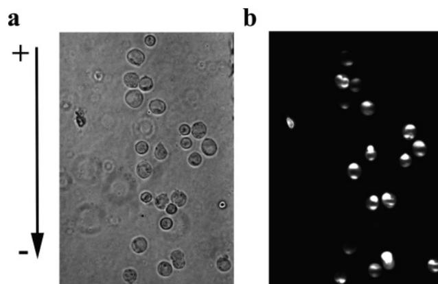
**Figure 4.** Electroporation of suspended CHO cells (before culturing) with a pulse of 30 ms and a pulse intensity of 209 V/cm. The channel contains 5 μM SYTOX green during the electroporation. The images were taken 5 min after the electroporation. (a) Phase contrast. (b) Fluorescence.
