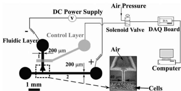
**Figure 1.** Design of the microfluidic electroporation device. The control channel (gray) is on top of the fluidic channel (black) with a PDMS membrane in between. The valve locates in the vertical fluidic channel 1, and the cell culture is in the horizontal fluidic channel 2. A common dc power supply is kept on during the operation of the device.
