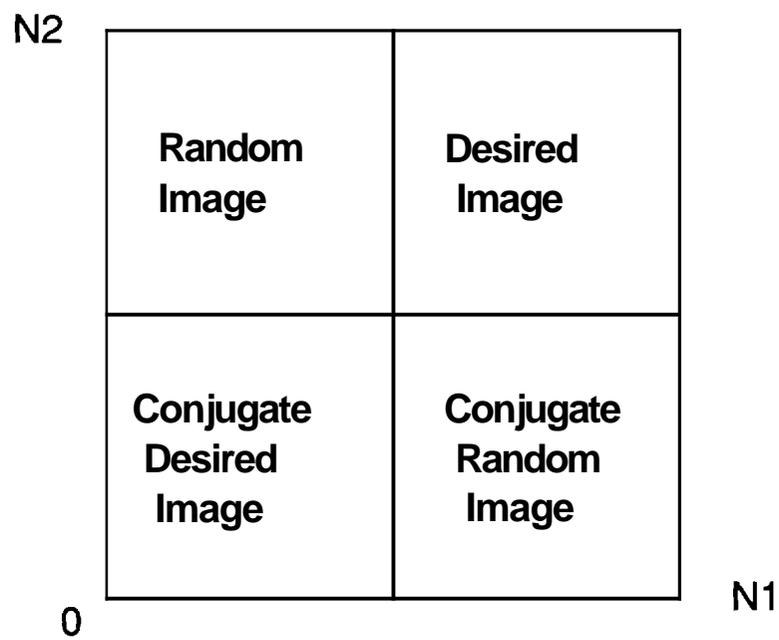
**Fig.1. Hermitian Symmetry Used in the POCS-CT Algorithm.**
