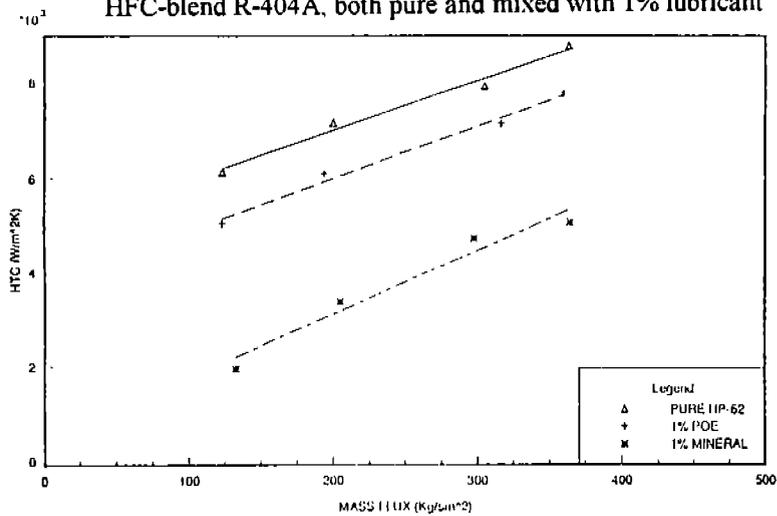
**Figure 5** Comparison of micro-fin tube evaporation heat transfer coefficients for HFC-blend R-404A, both pure and mixed with 1% lubricant
