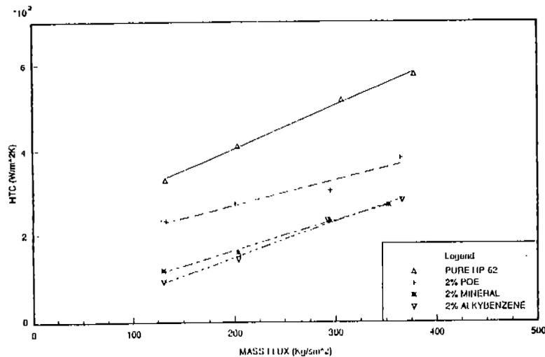
Figure 2 Comparison of smooth tube evaporation heat transfer coefficients for HFC-blend R-404A, both pure and mixed with 2% lubricant
