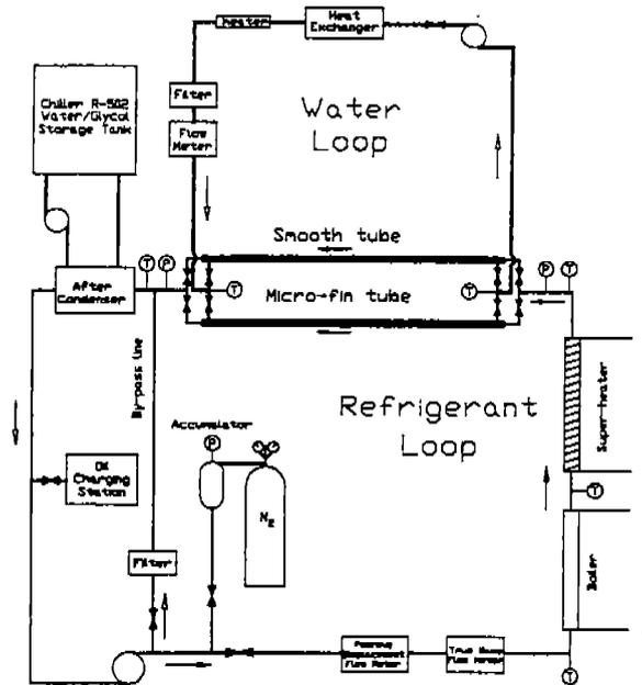
Figure 1 Schematic of in-tube evaporation test facility
