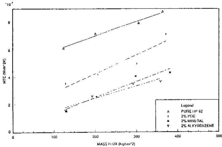
**Figure 3** Comparison of micro-fin tube evaporation heat transfer coefficients for HFC-blend R-404A, both pure and mixed with 2% lubricant
