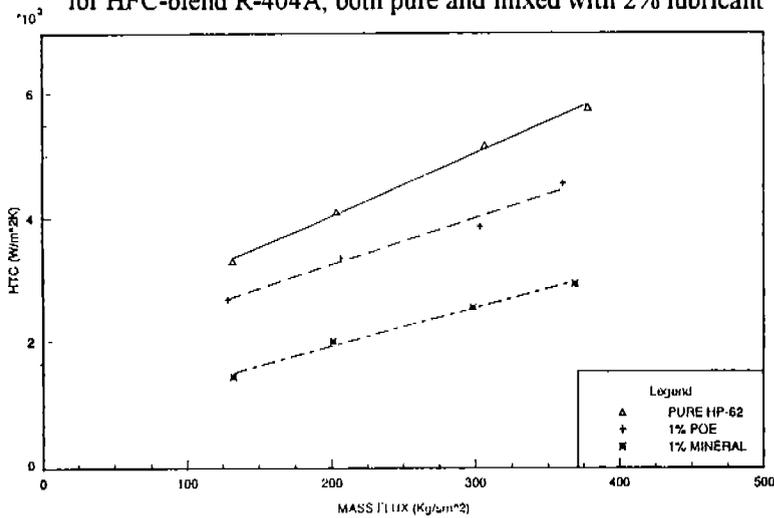
**Figure 4** Comparison of smooth tube evaporation heat transfer coefficients for HFC-blend R-404A, both pure and mixed with 1% lubricant
