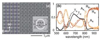
Fig. 1. (Color online) (a) Background shows the FESEM image of the NIM sample; the inset in Fig. 1(a) depicts the unit cell of the simulated structure. (b) Comparison of the experimental transmission  $(T_e)$ , reflection  $(R_e)$ , and absorption  $(A_e)$  spectra of the sample with simulated results  $(T_s, R_s, \text{ and } A_s)$  at the primary linear polarization as shown in Fig. 1(a).
