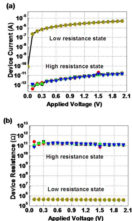
FIG. 3. (a) Measured  $I$ - $V$  characteristics and (b)  $R$ - $V$  characteristics of  $\text{In}_2\text{Se}_3$  nanowire memory, both plots showing four successive testing sweeps after nanowire was either set to low-resistance state or reset to high-resistance state.
