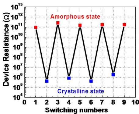
FIG. 4. Measured  $\text{In}_2\text{Se}_3$  nanowire device resistance for a series of high and low resistance states after repeated reset-set programming cycles. Device was switched from LRS to HRS using a 7 V/20 ns reset pulse (with 2 ns sharp fall-down edge), and from HRS to LRS using a 5 V/100  $\mu\text{s}$  set pulse.
