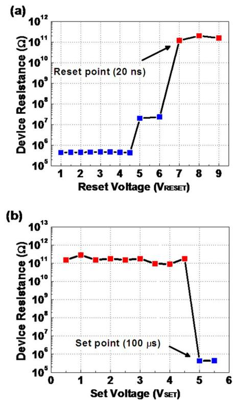
FIG. 2. Resistance of  $\text{In}_2\text{Se}_3$  nanowire memory (measured at a small read voltage of 0.2 V) as a function of applied voltage in a pulse-mode test. (a) Switching from low-resistance state to high-resistance state with a fixed pulse width of 20 ns. The reset starts to occur at 7 V. (b) Switching from high-resistance state to low-resistance state with a fixed pulse width of  $100 \mu\text{s}$ . The set starts to occur at 5 V.
