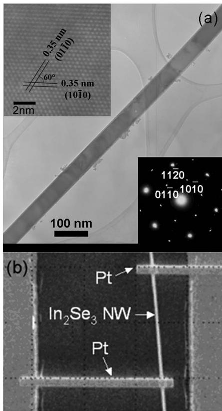
FIG. 1. (a) TEM image of an  $\text{In}_2\text{Se}_3$  nanowire grown on  $\text{SiO}_2$  substrate using 20 nm gold nanoparticles as catalyst. Top left inset shows the nanowire crystalline lattice structure and bottom right inset shows the SAED pattern. (b) Top view of the fabricated  $\text{In}_2\text{Se}_3$  nanowire memory device. Pt interconnection lines were deposited by focused ion beam, linking the  $\text{In}_2\text{Se}_3$  nanowire with prepatterned Mo probing pads.
