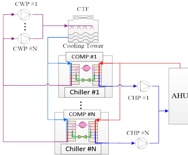
**Figure 2:** A chilled-water plant with  $N$  chillers in parallel.
