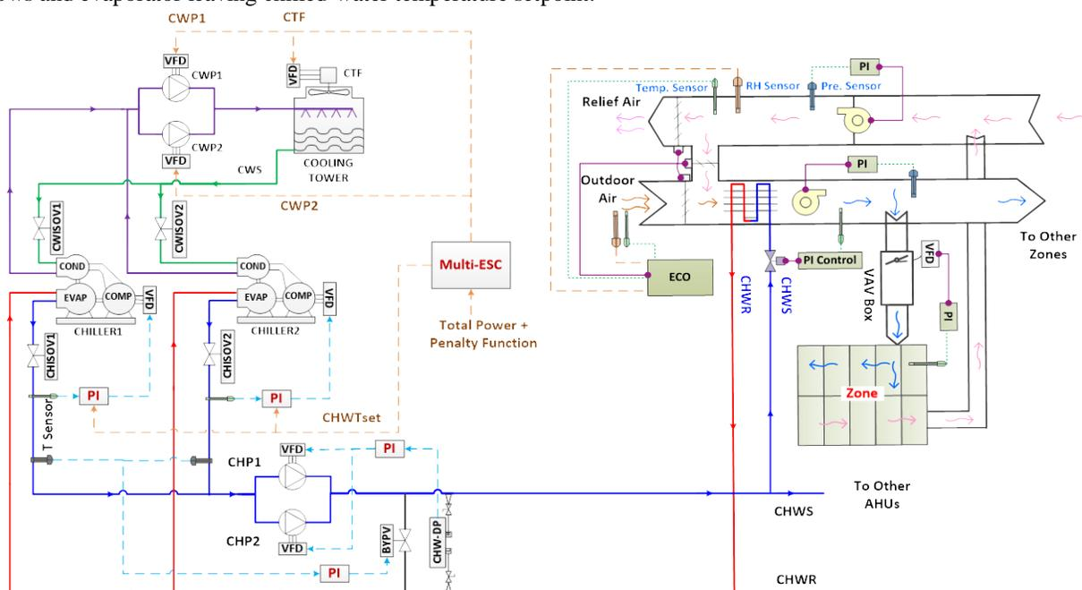
**Figure 1:** Schematic of a chilled-water plant with two chillers in parallel.
