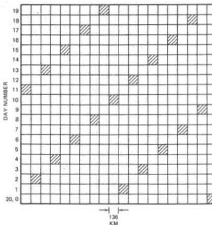
Figure 2. Coverage Patterns of Two Sun-Synchronous Orbits.
