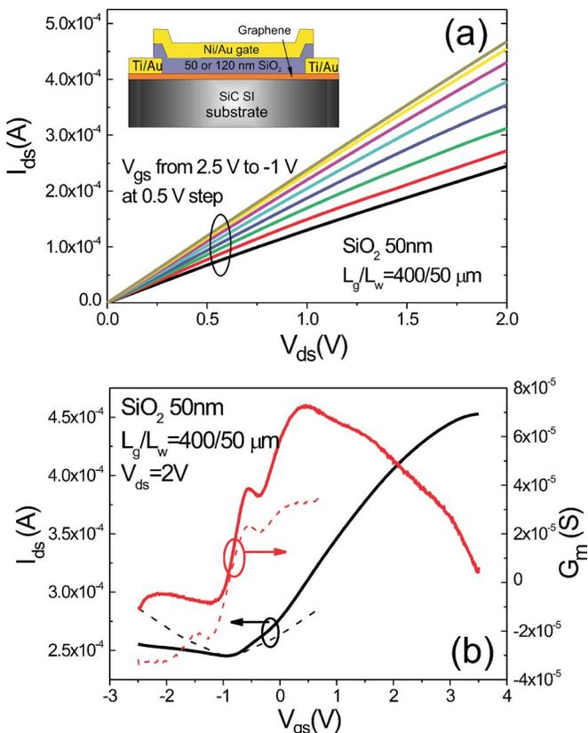
FIG. 2. (Color online) (a)  $I_{ds}$  vs  $V_{ds}$  as a function of  $V_{gs}$  on a few-layer graphene FET measured at room temperature.  $V_{gs}$  changes from  $2.5$  V (top) to  $-1.0$  V (bottom) in  $0.5$  V steps. (b) Transfer characteristics of the same device at  $V_{ds}=2$  V. The dashed lines are corrected one around Dirac point after extracting the  $p$ - $n$  junction resistance or “odd” resistance component (see Ref. 21).
