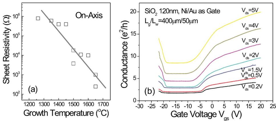
FIG. 3. (Color online) (a) Sheet resistivity of graphene films formed on SiC as a function of growth temperature. The gray line is a guide to the eye. (b) Drain conductance vs  $V_{gs}$  as a function of  $V_{ds}$  on a possible monolayer graphene FET measured at room temperature. The graphene film is formed on Si face of SiC. A clear  $n$ -type to  $p$ -type transition is obtained once the gate bias is strongly positive or negative.
