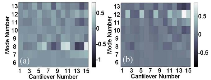
FIG. 3. (Color online) (a) Plot of the change in each eigenmode  $\Delta u_i$  before and after the addition of a 10 pg microsphere to cantilever 10. In this case, mode 8 undergoes the greatest change. (b) Plot of  $\Delta u_i$  before and after the addition of a 10 pg microsphere to cantilever 14. The greatest change is observed in mode 12 in this case.
