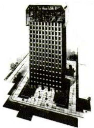
FIGURE 1 AUTOMATED CONSTRUCTION OF BUILDING (OHYASHI CORPORATION)
