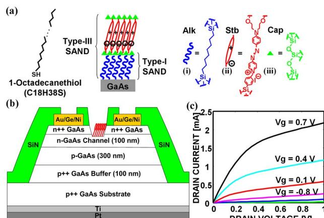
FIG. 1. (Color online) (a) Molecular structures of ODT, type-I SAND, and type-III SAND with components Alk, Stb, and Cap. (b) Cross-sectional view of a GaAs JFET (c) Output characteristic of a representative as-fabricated device.
