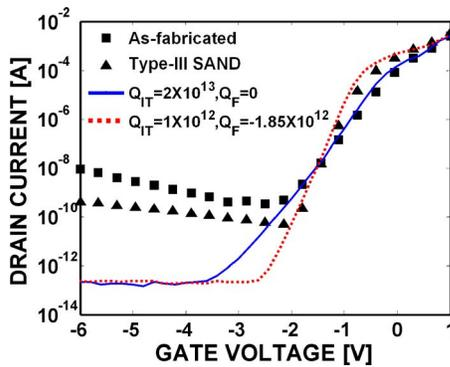
FIG. 3. (Color online) Transfer characteristics from experimental data for (i) as-fabricated (squares) and type-III SAND-modified (triangles) GaAs JFETs and (ii) MEDICI simulations for as-fabricated (solid lines) and type-III SAND-modified (dotted lines) GaAs JFETs. Fitting parameters are fixed surface charges ( $Q_F$ ) and interfacial traps ( $Q_{IT}$ ).
