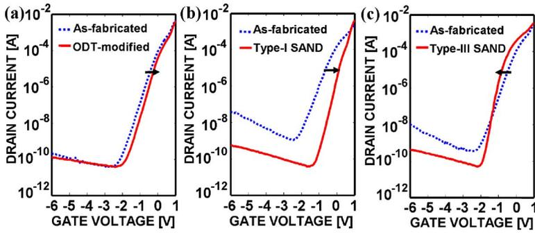
FIG. 2. (Color online) Transfer characteristics of GaAs JFETs modified with (a) ODT, (b) type-I SAND, and (c) type-III SAND. A negative threshold voltage shift ( $\sim 0.3$  V) with a steep subthreshold slope (178 mV/decade) is observed with type-III SAND passivation.  $V_{DS}$  was set to 0.1 V. The profiles of each subfigure refer to the same device.
