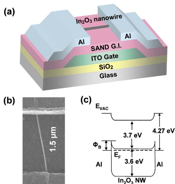
FIG. 1. (Color online) SAND-based  $\text{In}_2\text{O}_3$  NWTs. (a) Cross-sectional view of the device structure. (b) Top-view FE-SEM images of the device region. Scale bar = 1.5  $\mu\text{m}$ . (c) Source/nanowire/drain cross-section band diagram at  $V_{\text{gs}}=0 \text{ V}$ .
