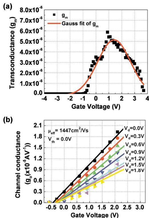
FIG. 3. (Color online) (a) Measured transconductance ( $g_m$ ) at  $V_{ds}=0.5$  V, along with a Gaussian fit to the data. (b) Measured channel conductance ( $g_d$ ) vs  $V_{gs}$ , with various curves corresponding to steps in  $V_{ds}$  from 0.0 to 1.8 V.
