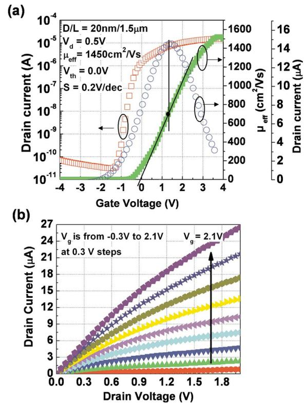
FIG. 2. (Color online) Measured characteristics of a representative SAND-based In<sub>2</sub>O<sub>3</sub> NWT. (a) Drain current versus gate-source voltage ( $I_{ds}-V_{gs}$ ) characteristics at  $V_d=0.5$  V. Green, red, and blue data points correspond to linear-scale  $I_{ds}-V_{gs}$ , log-scale  $I_{ds}-V_{gs}$ , and mobility  $\mu$ . (b) Drain current vs drain-source voltage ( $I_{ds}-V_{ds}$ ) characteristics for various values of  $V_{gs}$  ( $-0.3$  to  $2.1$  V in  $0.3$  V steps).
