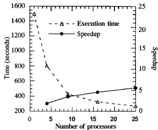
Figure 6. Results of experiment 7S. Simulation, using 4—25 transputers, of a network of 24x24 routers (25x25 for the case of 25 transputers) with 4-flit messages at load 50.
