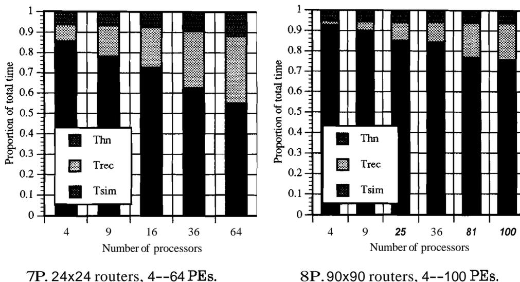
Figure 11. Distribution of total execution time among simulation and synchronization for experiments 7P and 8P. **Thn** = time spent computing the acceptance horizon and sending null messages; **Trec** = time spent receiving messages (null messages included); **Tsim** = time spent executing events and sending non-null messages.
