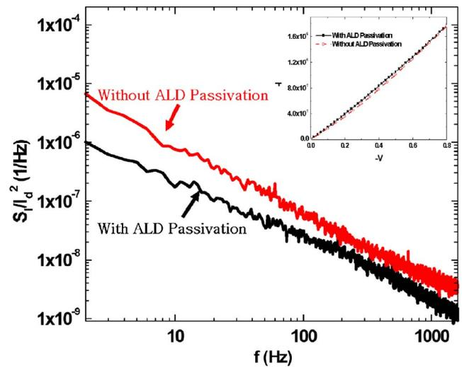
FIG. 2. Low frequency noise spectrum of current fluctuation of the pre-postpassivation of ALD  $\text{Al}_2\text{O}_3$  SWCNTs for drain to source resistor. Inset:  $IV$  characteristics of pre-postpassivated SWCNT. Both resistances have the same resistance of 500 k $\Omega$ .
