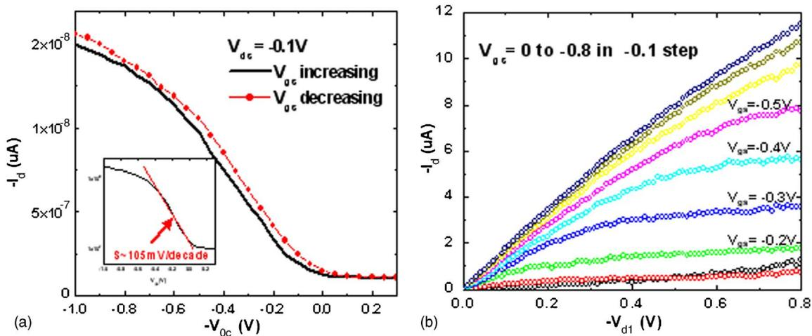
FIG. 4. Characteristics of a *p*-type SWCNT-FET with  $\text{Al}_2\text{O}_3$  as gate dielectrics. (a) Current  $I_d$  vs  $V_{gs}$  as increasing (line) and decreasing gating sweeps (points) for a  $1.5 \mu\text{m}$  gate-length SWCNT-FET at  $V_{ds}$  of  $-0.1 \text{ V}$ . Inset: log-scaled current  $I_d$  vs  $V_{gs}$  curve. The subthreshold swing ( $S$ ) is about  $105 \text{ mV/decade}$ . (b) Drain current vs drain bias as a function of gate bias of the same device.
