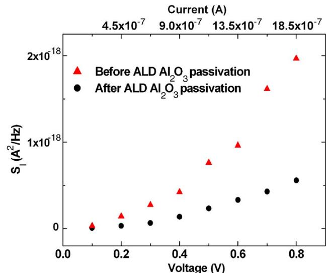
FIG. 3. Current vs current noise amplitude of  $S_I$  for drain to source resistor at 10 Hz as a function of voltage prior to ALD  $\text{Al}_2\text{O}_3$  passivation and after ALD  $\text{Al}_2\text{O}_3$  passivation.
