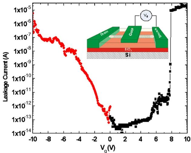
FIG. 1. Leakage current  $I_g$  (A) vs gate bias  $V_g$  (V) for SWCNT-FETs having 15 nm  $\text{Al}_2\text{O}_3$  dielectrics. Inset: cross section of the top gate single-walled carbon nanotube field effect transistors with 15 nm thick ALD-grown  $\text{Al}_2\text{O}_3$  as gate dielectric.
