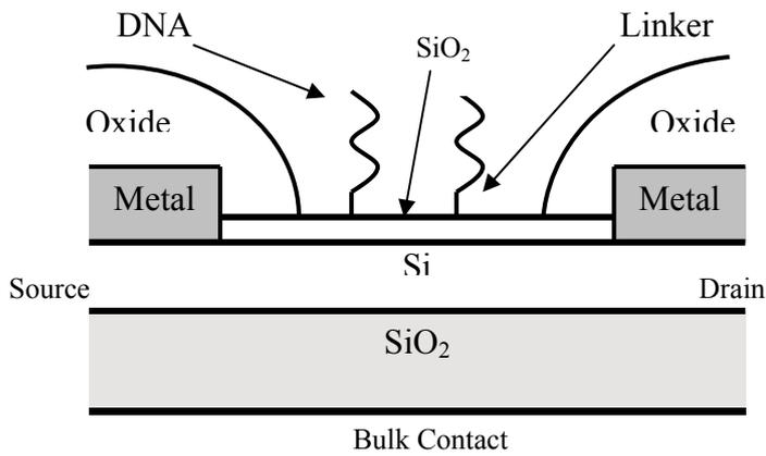
Figure 1. This is a schematic diagram of the conventional SOI DNAFET structure. The DNA molecules are bound to the SiO<sub>2</sub> surface layer by an uncharged linker molecule.
