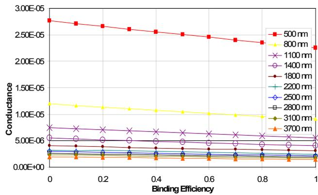
Figure 2. Conventional structure simulation with a probe spacing length of 10 nm and a surface oxide thickness of 4 nm. The absolute values of the conductance were calculated, and for smaller devices the relative change in conductance was greater than that for larger-sized devices.
