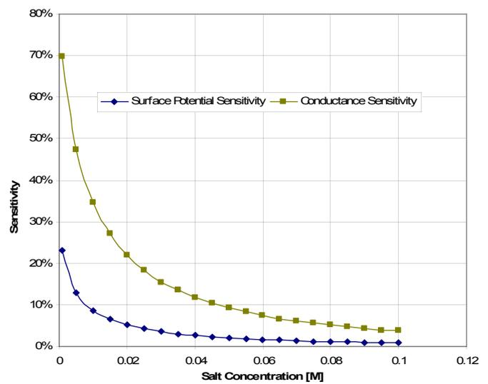
Figure 4. Conventional structure simulation with a probe spacing length of 10 nm and a surface oxide thickness of 4 nm. The conductance and surface potential were calculated in two states; initially with only the probe molecules attached to the surface and then with the probe molecules bonded with the target molecules. Sensitivity is defined as the difference between the values with two strands and the potential with one strand divided by the value with one strand.
