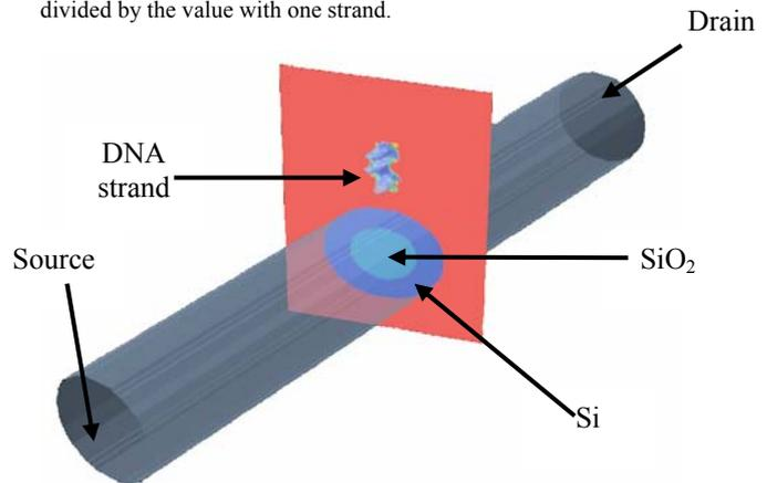
Figure 5. Silicon nanowire DNAFET diagram.
