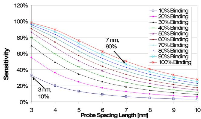
Figure 3. Conventional structure simulation with a sensor length of 3 and a surface oxide thickness of 4 nm. 0% binding is calculated with only probe molecules attached to the surface. The baseline is the 0% binding level. Sensitivity is defined as the difference between the conductance with two strands and the conductance with one strand divided by the conductance with one strand.
