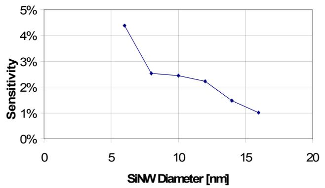
Figure 6. Silicon nanowire structure simulation with a channel length of 20 nm and a surface oxide layer thickness of 2 nm.
