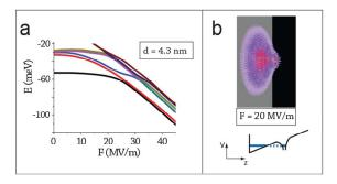
**FIGURE 2.** a) Eigenlevels (E) of an As donor 4.3 nm below a  $SiO_2$  interface as a function of electric field (F) calculated in NEMO-3D. b) Wavefunction density of the ground state of an As donor at d=4.3 nm and F=20 MV/m. The gray plane represents the  $SiO_2$  interface. The ground state is a hybrid combination of donor-like and well-like states.
