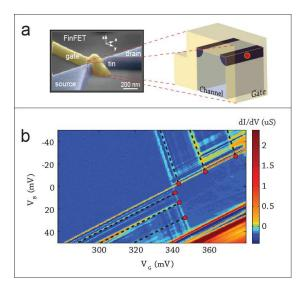
**FIGURE 1.** a) Colored Scanning Electron Micrograph of a FinFET device. Blow-up schematically shows channel/gate with current-carrying region (dark-blue) and donor atom (red dot). b) Stability diagram of a typical D<sup>0</sup> charge state. The dashed black lines indicate the presence of excited eigenlevels..
