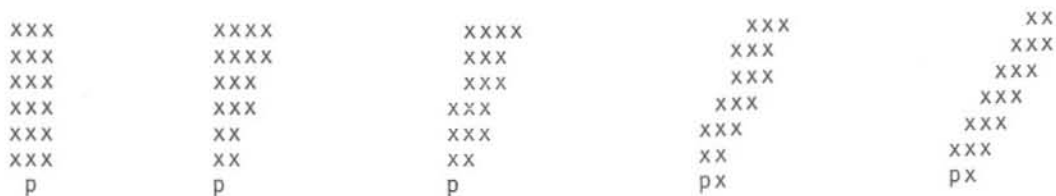
Figure 13. Masks used in Version II of the line orientation alignment algorithm.
