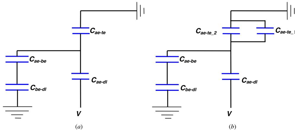
**Figure 3.** Capacitive network for the estimation of voltages across the capacitive elements: (a) analytical approach 1 and (b) analytical approach 2.
