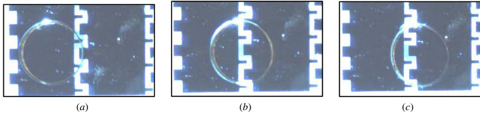
**Figure 5.** Electrically induced transition of a transformer oil droplet at (a)  $t = 0$  s, (b)  $t = 0.8$  s and (c)  $t = 1.73$  s (the grounded electrode is on the left and the actuated electrode is on the right).
