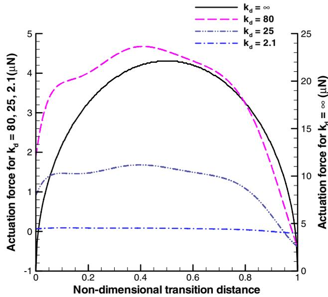
**Figure 8.** Electrical actuation force dependence on droplet dielectric constant at an actuation voltage of 50 V. The y-axis on the right of the plot is used to represent the curve for  $k_d = \infty$  for the improved resolution.
