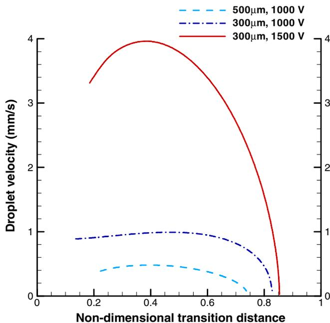
**Figure 10.** Measured droplet velocities for an electrically actuated transformer oil droplet at different plate spacings and actuation voltages.
