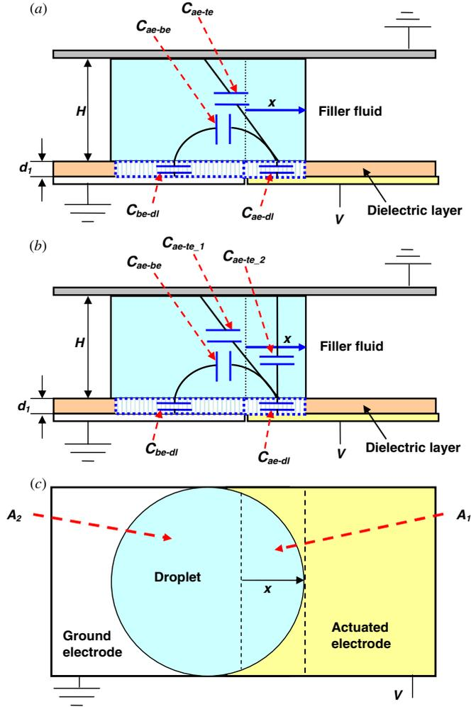
**Figure 2.** Schematic illustration of a droplet undergoing transition: (a) side view showing analytical approach 1, (b) side view showing analytical approach 2 and (c) top view.
