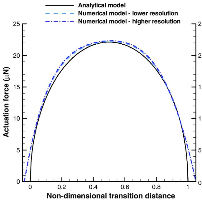
**Figure 6.** Comparison of analytical and numerical model predictions.
