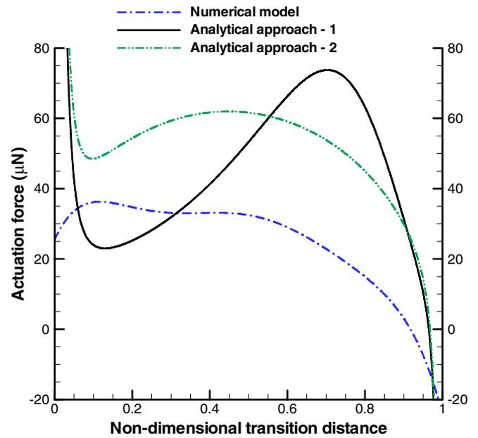
**Figure 7.** Electrical actuation force prediction using analytical and numerical models for a 1 mm radius transformer oil droplet ( $k_d = 2.1$ ) at an actuation voltage of 1000 V.
