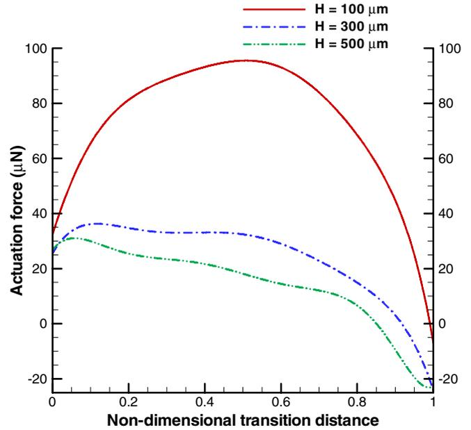
**Figure 9.** Electrical actuation force dependence on plate spacing for a 1 mm transformer oil droplet ( $k_d = 2.1$ ) at an actuation voltage of 1000 V.
