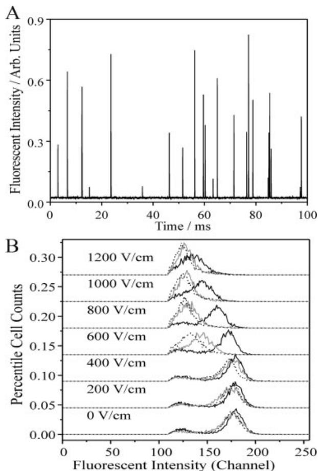
**Figure 3.** (A) Fluorescent intensity over time recorded by the photomultiplier tube when calcein AM-loaded DT40-Syk<sup>-</sup> cells flow through the device. (B) Histograms of fluorescent intensity generated by calcein AM-loaded DT40-Syk<sup>-</sup> cells under different electric field intensities and different durations (black, 50 ms; gray, 100 ms; dot line, 150 ms).
