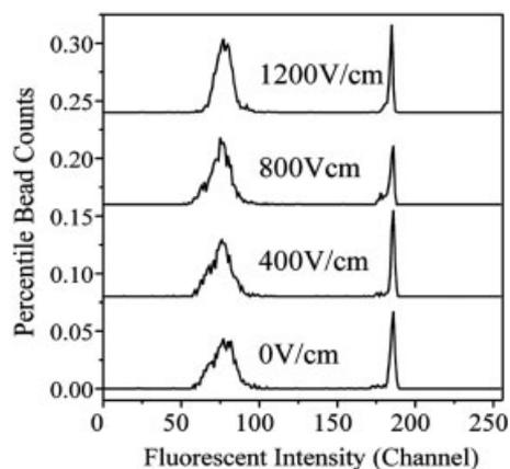
**Figure 2.** Histograms of fluorescent intensity generated by mixed microspheres ( $D \sim 10$  and  $1 \mu\text{m}$ ) under different electric field intensities in the narrow section taken using the device in Fig. 1 in the main text.
