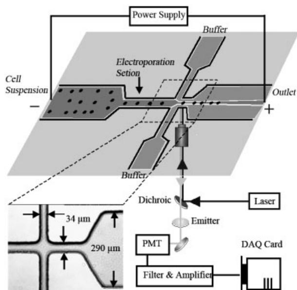
**Figure 1.** Schematic of the microfluidic system for the electroperative release of intracellular materials at the single-cell level. The details about the setup and the data collection are given in Section 2.
