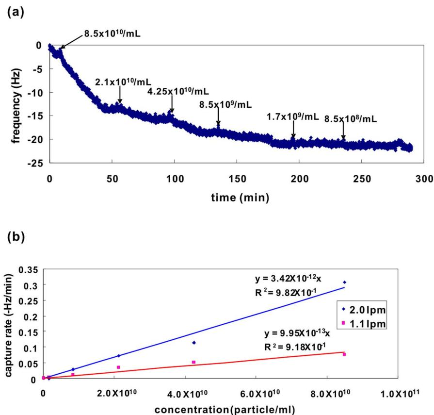
FIG. 3. (Color online) (a) Real-time measurements with different concentrations ( $8.5 \times 10^8$ – $8.5 \times 10^{10}$  particles/ml) of virus suspension where *Vaccinia* viruses were captured on a QCM crystal at a flow rate of 2.0 l/min. (b) Variation of capture rate of *Vaccinia* viruses with different virus concentrations ( $8.5 \times 10^8$ – $8.5 \times 10^{10}$  particles/ml) at flow rates of 1.1 and 2.0 l/min. The lines indicate linear fits.
