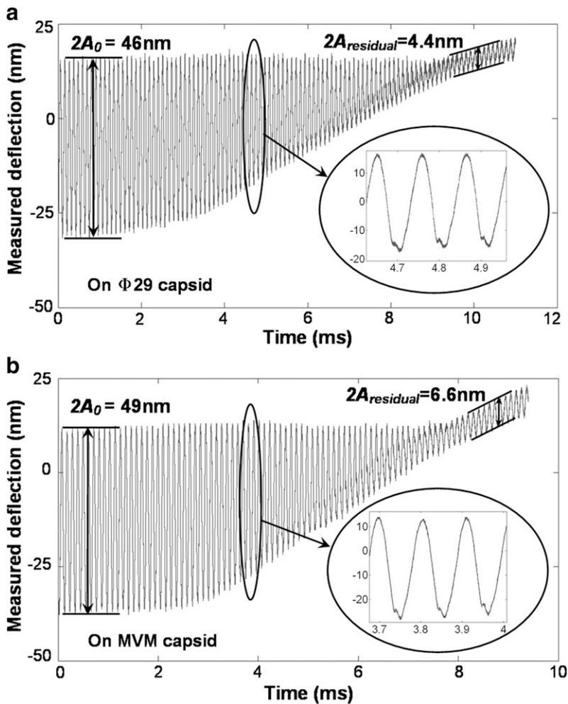
FIGURE 3 Waveforms acquired from experimental approach curves using the SL probe made on top of (a)  $\Phi 29$  (b) MVM virus capsids. The characteristic distortion of the deflection signal caused by intermittent contact with the sample can be clearly seen from the inset figure. Moreover, the dither piezo motion  $A_{\text{residual}}$  is much smaller compared to the free amplitude of the tip, at least for large amplitude setpoints that are typically used for imaging.
