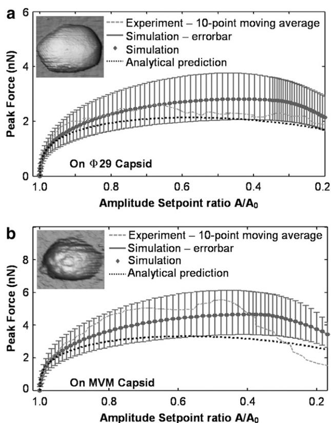
FIGURE 6 Peak interaction forces on (a)  $\Phi 29$  and (b) MVM with inset of AFM images. The dashed curves are experimental data extracted by the acceleration method (smoothed using 10-point moving average), the point/solid curves are predictions from mathematical simulations using Eqs. 1 and 4 along with the error bars (standard deviation), and the dotted curves are the analytical prediction using Eq. 9 using parameters in Table 3.
