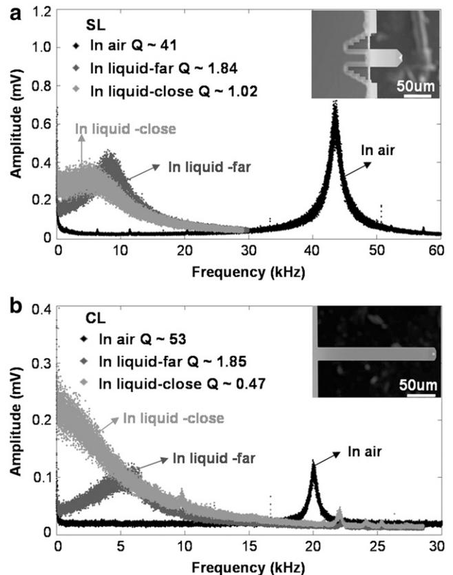
FIGURE 5 Thermal spectrum (Brownian motion excited) of SL and CL in air and liquid far and close to the surface. The values of the  $Q$  factor are indicated in the graphs. (a) Thermal spectrum for SL is represented showing the decrease of the  $Q$  factor in liquid when it is close to the sample. (b) Thermal spectrum for CL is represented showing the overdamped behavior when it is close to the surface.
